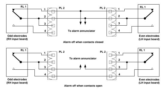
(Switch SW5 is set to ES for low level alarms and set to EW for high level alarms)
